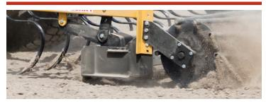
Every MK Martin Track Curry comes with two standard spill plates. These funnel any excess material into the Track Curry's path, ensuring your arena or track keeps looking its best.
