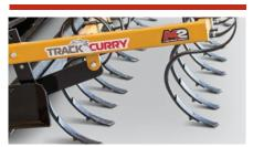
The two rows of S-tines works to loosen the material in your riding arena bringing the lower layer material to the top as they pull through ground. The S-tines are equipped with replaceable tips for easy maintenance and optimum performance.
